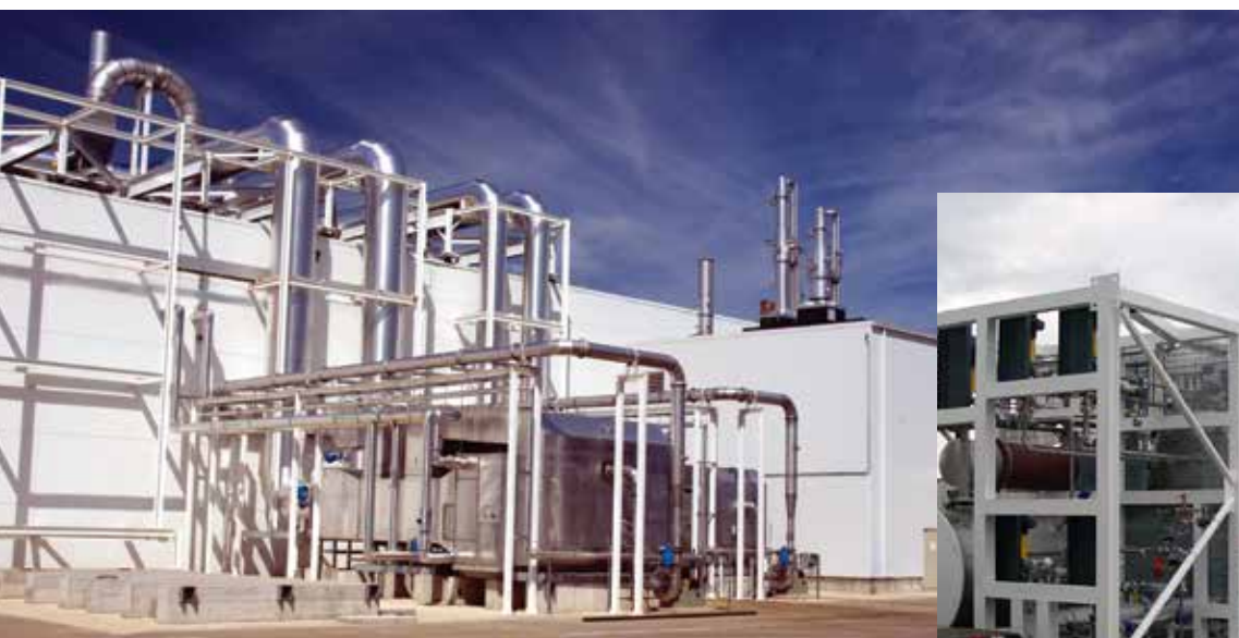
All Dürr MEGTEC distillation and purification systems can be supplied pre-assembled on skids for timely and easy installation.
