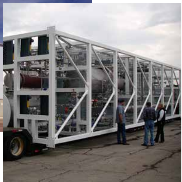
All Dürr MEGTEC distillation and purification systems can be supplied pre-assembled on skids for timely and easy installation.
