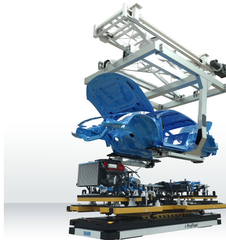
During the marriage process, drive and chassis components (engine, motor, gearbox, battery, axles, etc.) are combined with the accompanying body
