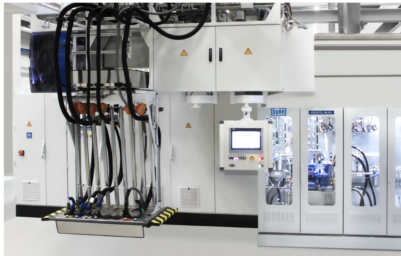
Combined filling of all media types with one ProLine filling machine
