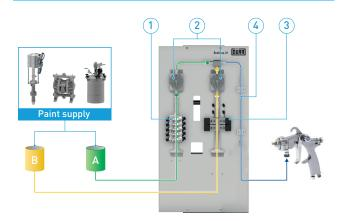
$\begin{array}{l} 1 \ \ Color \ change \ block \ component \ A, \ 2 \ \ Flow \ control \ / \ Measuring \ cell \ component \ A \ \& \ B \\ 3 \ \ Color \ change \ block \ component \ B, \ 4 \ \ Static \ mixer \ component \ A \ \& \ B \end{array}$
