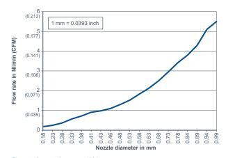
Flow rate for water / pressure 100 bar
